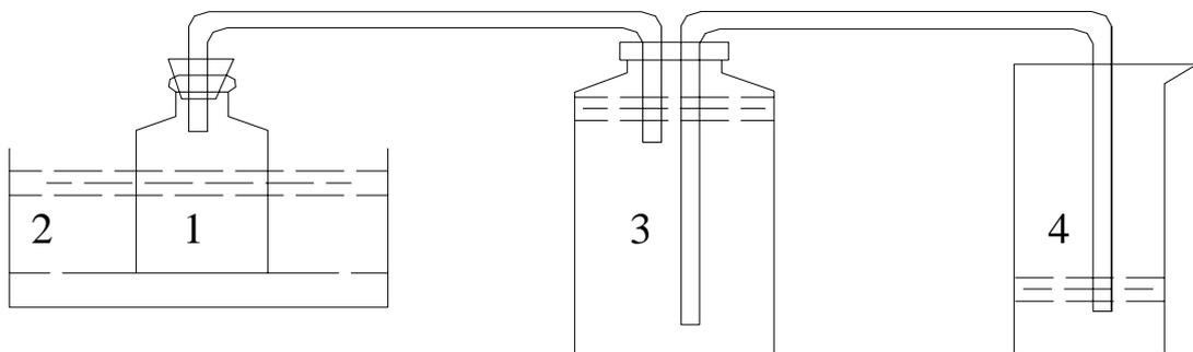
**Figure 1: Sketch of lab-scale digester and biogas collection apparatus used in the laboratory experiment (1—1 l Glass flask (Digester), 2—Thermostat water bath, 3—2 l Glass container (collecting biogas), 4—Measuring cylinder)**
